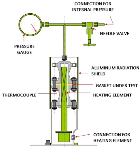
**Figure 6.** Thermal cycle test rig schematic
