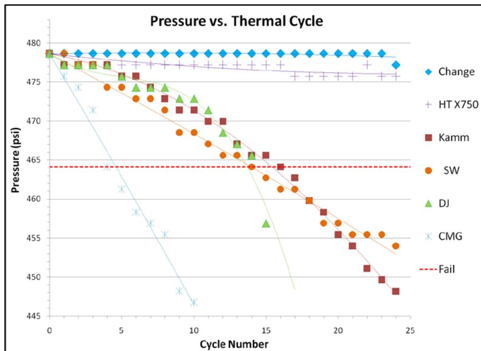
**Figure 8.** Thermal Cycle Test Results - 24 cycles to 320°C (608°F)
