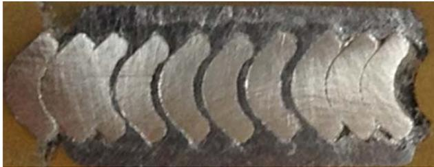
**Figure 2.** Change gasket cross sectional cutaway showing construction: wound like a spiral wound, faced like a kammprofile
