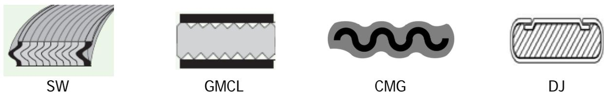
**Figure 1.** Typical cross section of semi metallic gaskets.
