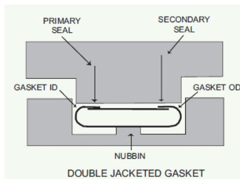
**Figure 9.** Tongue-to-groove joint with stress raising nubbin and a double jacketed gasket
